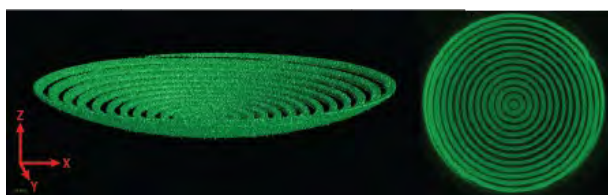
Figure 1: 3D (left) and top down (right) visualization of a concave hemisphere ( \kappa=1/1000 \mu\text{m}^{-1} ) containing a circular pattern (lines: 20 \mu\text{m} wide and 20 \mu\text{m} gaps) of gelatin-fluorescein (green).
